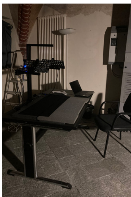
Helen Davies's smaller multispectral imaging system designed by the Rochester Institute of Technology and supported by a grant from the NEH.
